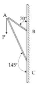
Suppose the force  $\overrightarrow{P}$  is resolved parallel to the arms AB and AC of the frame. The magnitude of the resolved component along the arm AC is x N. The value of x, to the nearest integer, is [Given :  $\sin(35^\circ)=0.573, \cos(35^\circ)=0.819$  $\sin(110^\circ)=0.939$ ,  $\cos(110^\circ)=-0.342$ ]
