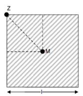
$$egin{aligned} I_z &= I_{cm} + Migg(rac{l}{\sqrt{2}}igg)^2 \ &= rac{Ml^2}{6} + rac{Ml^2}{2} = rac{4Ml^2}{6} = rac{2Ml^2}{3} \end{aligned}$$
